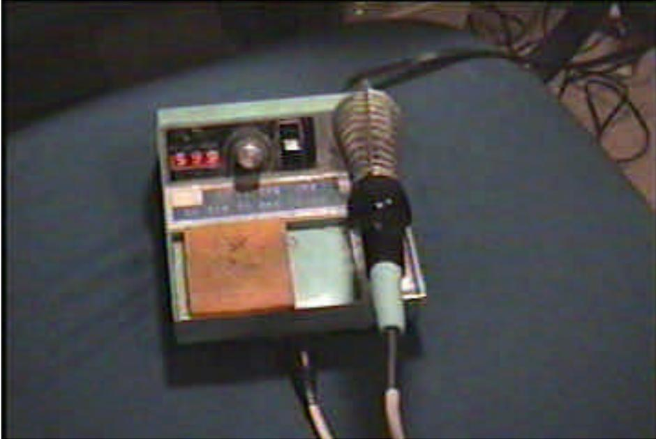
Quality soldering station made by Weller (Cooper Tools)
