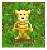
Another way of achieving this would have been to add semi-transparent pixels on the edges, but this implies using alpha-blending, which is not supported on all machines
